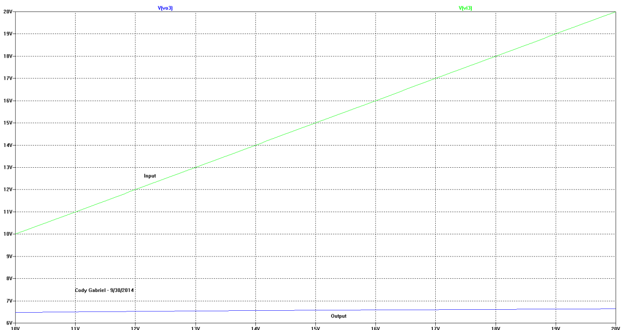
Figure 9: Input and output of Zener diode regulator circuit.
